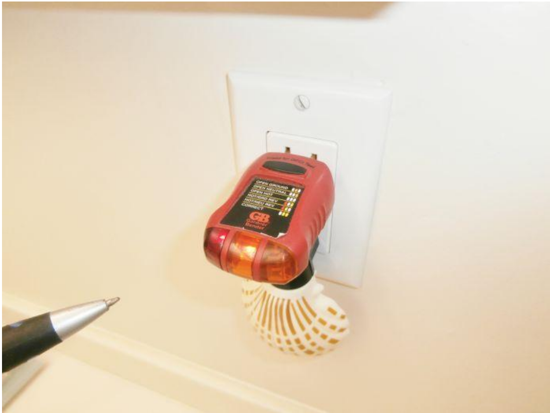
Bathroom #2 Hall downstairs / GFI(s)/Hot Neutral reverse
